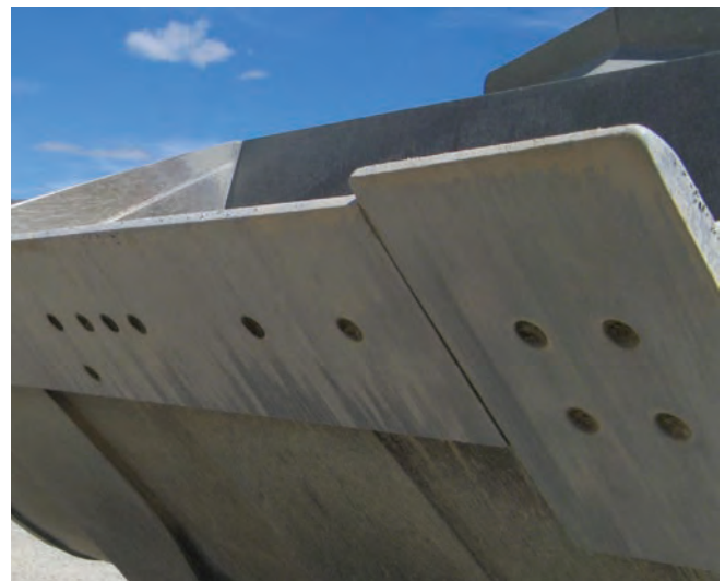
Bolt-on Cutting Edges
