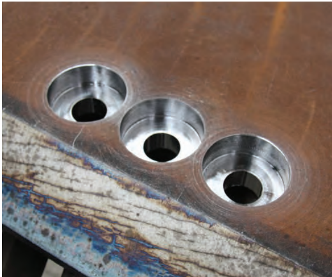
Drilled & Counterbored Holes
