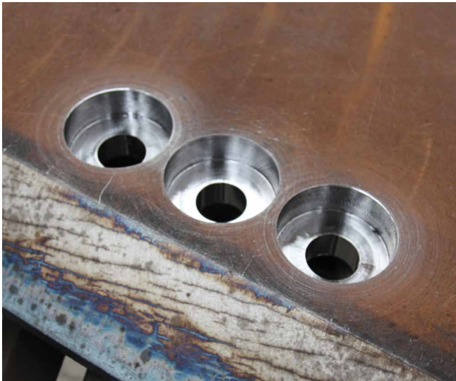
Drilled & Counterbored Holes
