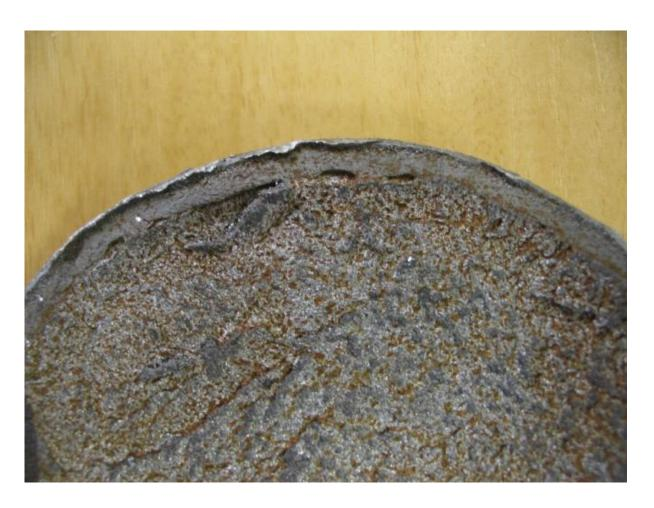
This failed shaft material had a high Ceq of 0.55, which means that it is essential that the parts are properly preheated for welding, and fully PWHT (stress-relief / temper) after welding.
