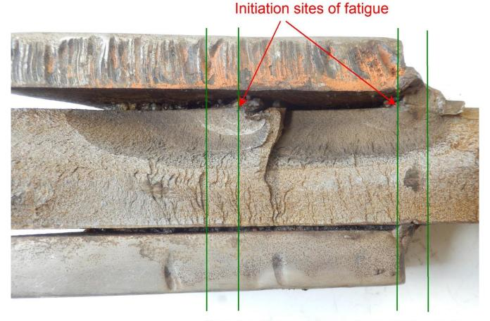
Cuts to allow sections for metallography
