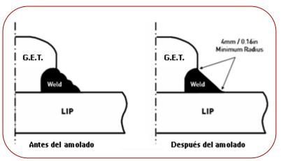
Grinding shall be done using high speed electric or pneumatic grinders with grinding wheels no larger than 50mm / 2.00 in. in diameter. ANGLE HEAD OR DISK GRINDERS ARE NOT ALLOWED FOR THIS WORK.
