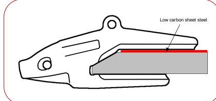
Alternatively the upper leg adapter may be built up by welding to acceptable dimensions in the follow manner:
