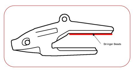
4. Grind weld so that there is a smooth transition in the weld
