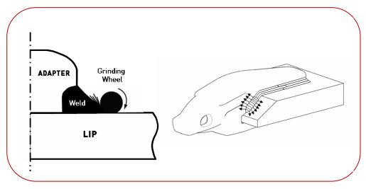
Proper Grinding Directions:
