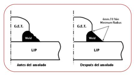
diameter. ANGLE HEAD OR DISK GRINDERS ARE NOT ALLOWED FOR THIS WORK.
