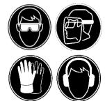
To avoid eye injury, always wear safety goggles or a protective mask when using any equipment, hammer or similar tool. When equipment is under pressure or when objects are struck, chips or other debris can be thrown out. Make sure no one gets hurt by the debris that is fired before applying pressure or hitting an object. Wear eye protection that complies with ANSI Z87.1 and OSHA standards. Also wear hearing protection and gloves.
