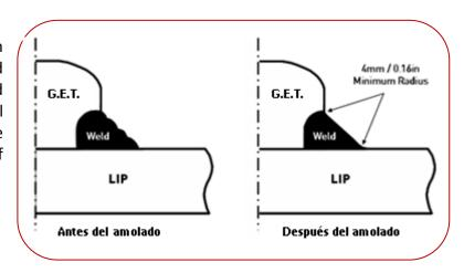
Grinding shall be done using high speed electric or pneumatic grinders
