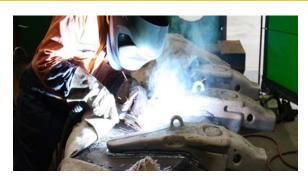
Weld must be done with short beads and a maximum oscillation of three times the diameter of the electrode. Completely remove the slags and lightly hammer the bead to reduce tensions after each run.
