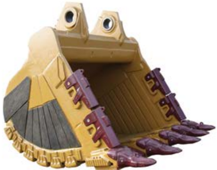
5130 Rock Bucket with StarMet Teeth, ProMet Lip and Side Protection, Chock Block and Wear Strips
