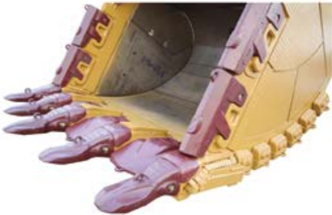
5130 Rock Bucket with StarMet Teeth, ProMet Lip and Side Protection, Chromium Carbide Liners and Bolt-on Heel Shrouds
