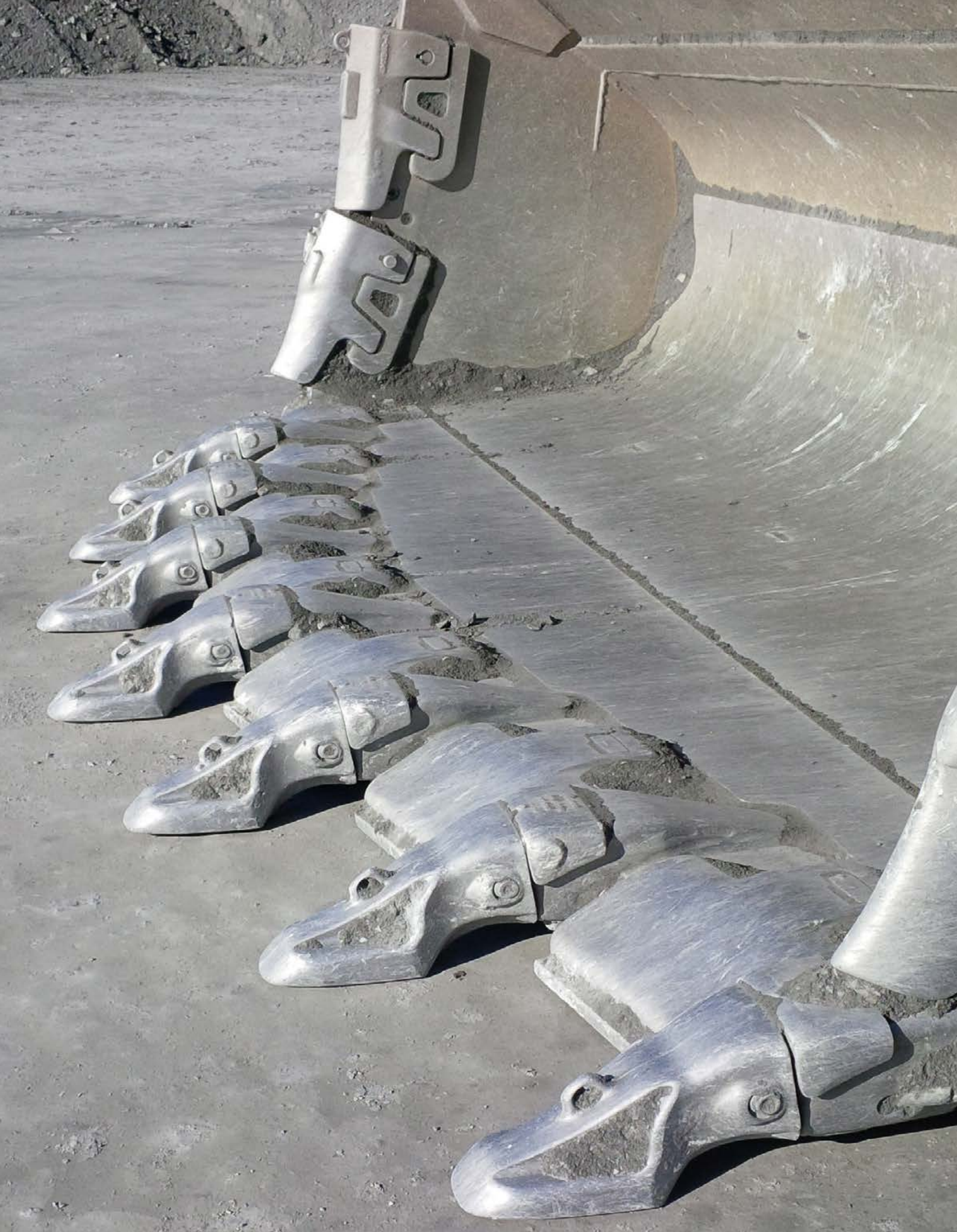
992 Loader Bucket with a fully hammerless GET wear package
